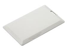
The MarkTag Classic read-only 2.45 GHz RFID Tag is a long—time proven high-end choice for hands-free vehicle identification. Each ID-tag has a pre-programmed 8-digit unique identity code. This Tag also has a large 32-bit checksum that virtually eliminates the risk of incorrect tag reads even in environments where several ID-tags are simultaneously being identified.
